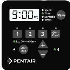
Figure 7: Activating External Control Only
