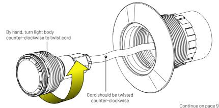
**6** - Insert the MicroBrite light into the 1.5" wall fitting. By hand start the process of threading the male threads on the MicroBrite's white threaded adaptor ring into the female threads of the wall fitting.
