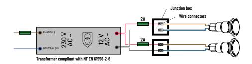
Maximum wattage using multiple lights (with a 300 Watt isolation transformer). IMPORTANT! When using multiple 12 VAC Pentair pool and spa lights the total allowable light wattage should not exceed 80% of rated value.
